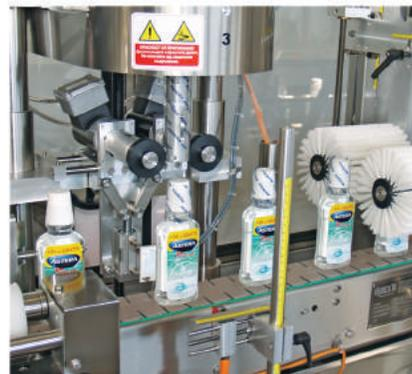
Machines for application of partial, full-body or tamper-evident thermo-shrinkable sleeve label. As an option they can be equipped with a perforating device for easy opening.
